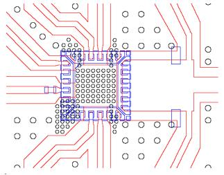
We recommend that all N/C pins be grounded and sufficient number of vias to be present under the ground plane. Pins 13 and 18 are connected to the RFout trace.
